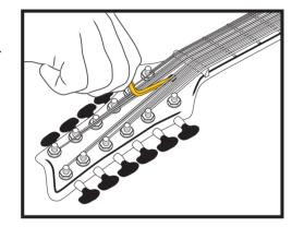
Turn clockwise (right) to reduce relief and flatten the neck — useful if the action feels high in the middle of the neck.
